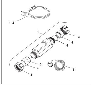
Figure 19. 2" PVC Union, Electrolytic Cell and DC Cable
