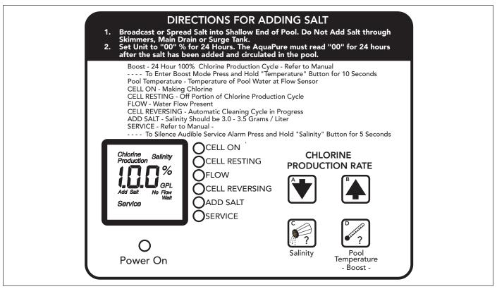
Figure 13. Control Center Front Panel
