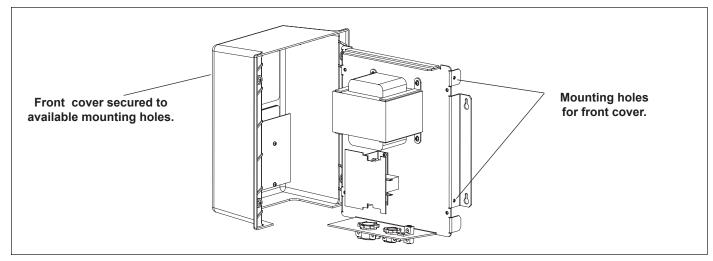
Figure 7. Securing the Control Center Front Cover to the Chassis Backplate
