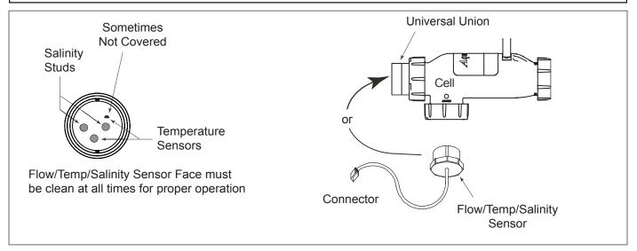
Figure 8. Flow/Temp/Salinity Sensor
