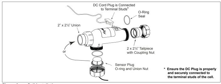
Figure 9. Cell Installation
