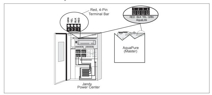
Figure 12. Wiring an AquaPure to an AquaLink RS Control System Network
