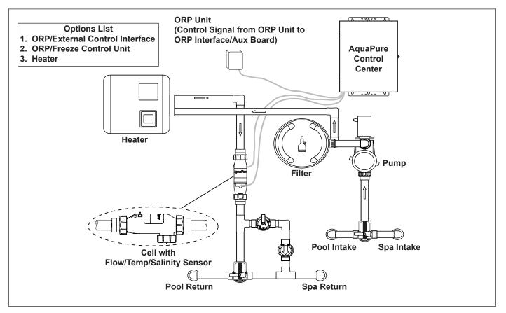
Figure 1. Typical AquaPure Installation With Options
