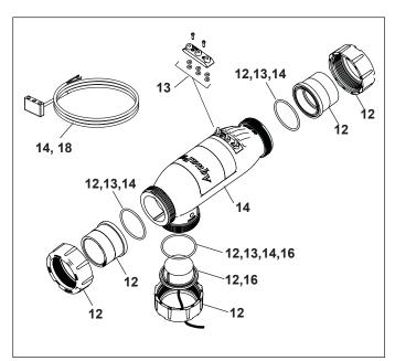
Figure 17. 3-Port Electrolytic Cell and Sensor Exploded View
