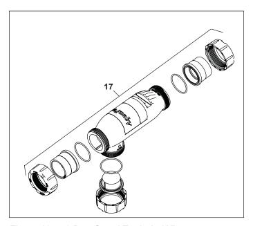
Figure 18. 3-Port Spool Exploded View
