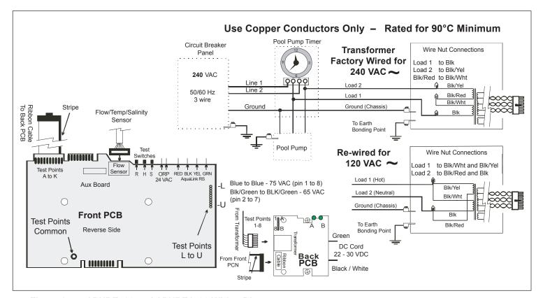
Figure 2. APURE700 and APURE1400 Wiring Diagram
