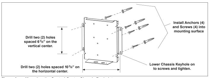
Figure 6. Mounting the Control Center Chassis Backplate
