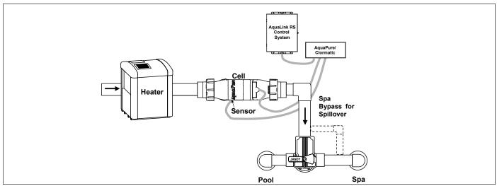
Figure 4. Recommended Plumbing Configuration for Pool/Spa Combination Systems
